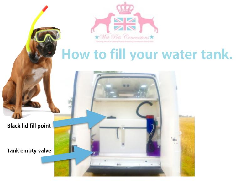
In the rear of your van is the fresh water tank. This is what supplies your Hydrobath with all of the fresh water that you need for the day. This is pumped via the water pump, into the rinse tank of your Hydrobath where it is heated by the Hydrobath heat element (unless you have a diesel heater fitted - in which case it is heated by the diesel heater and enters the rinse tank already heated).
